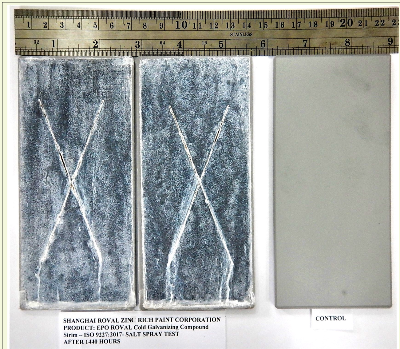
Scribed test sample of EPO ROVAL Cold Galvanizing Compound (ER96%) after neutral salt spray test at 1440 hours
